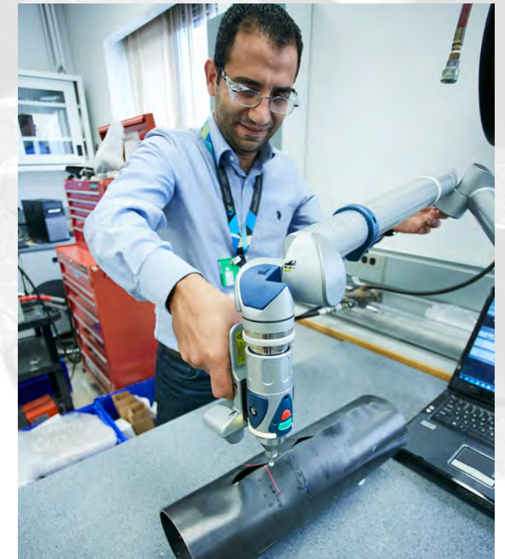
A CNL employee analyzes a sample of a bursted pressure tube as part of fuel channel research work for COG. The research has contributed to continued operation at Pickering and allowed for effective synchronization of the Darlington Refurbishment and Bruce Power MCR projects. Photo courtesy of CNL.
