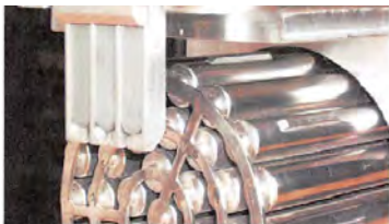
Figure 3: Close-up of finger tool on bundle showing latching device.
