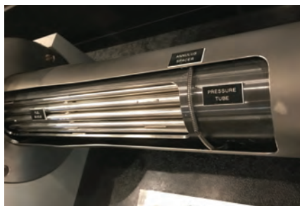
A cutaway from a fuel channel model shows the bundle within the tube with the annulus spacer
