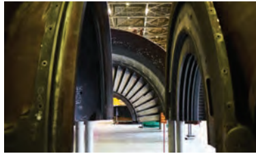
Far left: The Darlington turbine hall. For the first time all turbine blades and rotors were removed and reinstalled to ensure continued operation for another 30 years
